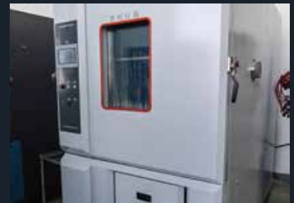
Climatic Test (climatic and thermal chamber)
